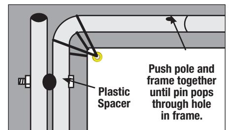
3. Align the pre-drilled holes on the assembled frame to the holes on one end post (C). Position a black plastic spacer (D) between the post and the frame. Slide one bolt (E) through the frame, spacer and post and secure with a nut (F). Repeat on other hole and with other post.
