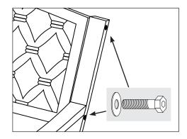
**3.** Align the holes on the back panel (C) with the holes in the legs (A) and secure using a 55mm bolt (E) and a washer (F). Repeat on other side. Set bench level on floor and adjust until all four legs are flush and square.
