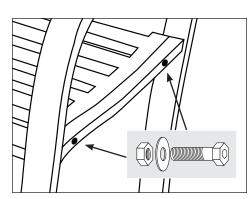
**2.** Use the provided wrench (H) to attach one leg frame (A) to one end of the seat panel (B). Slide a 50 mm bolt (D) through a washer (F) and the aligned holes and secure with a nut (G). Repeat with the other leg. Attach the nuts, but do not tighten completely until the entire bench is assembled and sitting square on the floor.
