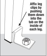
**4.** Optional: To Surface Mount, attach bench to concrete surface by clipping a leg clip (J) to the tabs on the inside of each leg. Determine your bench location and drill 4 holes into the concrete. Unscrew bolts from concrete anchors (F) and insert anchors into the holes. Position leg clips over each hole and insert bolts through the clips and into the anchors in the concrete. Tighten bolts to fully secure.
