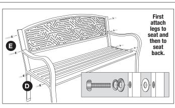
**2.** Use the provided wrench (K) to attach one leg frame (A) to one end of the seat panel (C). Slide a screw (E) through a lock washer (I), then a metal washer (G) and through the hole in the leg. Slide the plastic washer (H) between the leg and the seat panel before finally tightening the screw into the seat. Repeat with the other leg. Do not tighten completely until the entire bench is assembled and sitting square on the floor.
