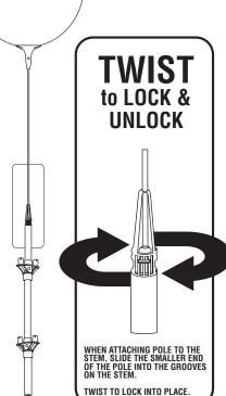
\*REPEAT STEP FOR ALL REMAINING STEM HANDLES AFTER THEY **ARE ASSEMBLED ONTO** REMAINING PLASTIC FITTINGS.
