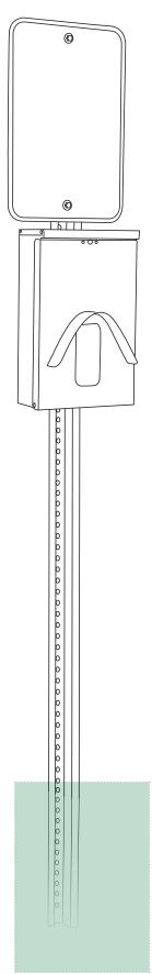
Using a post hole driver (not included), drive the sign post (C) approximately 15-18" into the ground. Make sure that the "hollow" or "recessed" side of the post is facing where you want the front of the unit to face. Use a level (not included) to ensure the pole is standing upright and will properly support the unit. Adjust if necessary.
